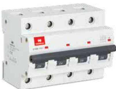
Higher Rating FP MCB (80 A-125 A) 'C' Series, (In accordance with IS/IEC 60947-2) 240 V/415 V, 50 Hz, 10 kA
