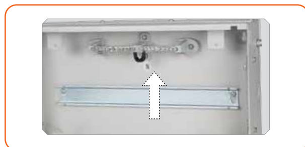
Remove link to use split neutral provision • Use 1st neutral link for mains supply • Use 2nd neutral link for stand by supply
